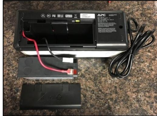
1. Remove battery by sliding cover off of bottom of the unit.
