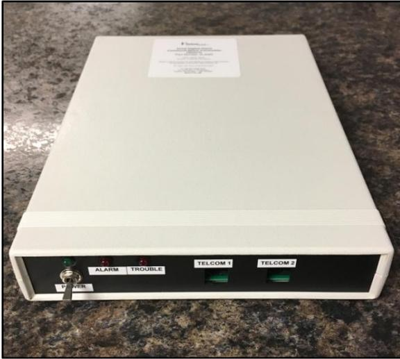
*NOTE: The SDACT dialer will need to be programmed on site with monitoring station account information. The software required is located on the flash drive provided in the Support folder under SDACT Keltron Programmer.*
