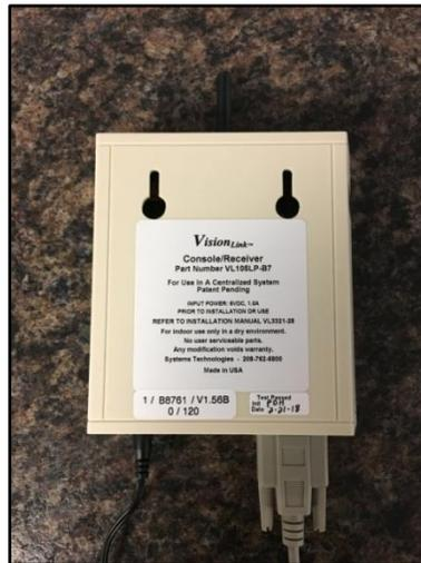
*NOTE: Install console receiver a minimum of 4 ft. away from other electronic equipment and other metal surfaces.*
