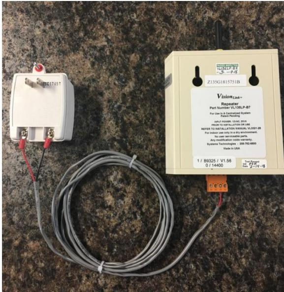
*NOTE: All types of repeaters have a maximum 75 ft.-radius coverage area. These repeaters need to be spaced no more than 150 ft. from other repeating/receiving units.*
