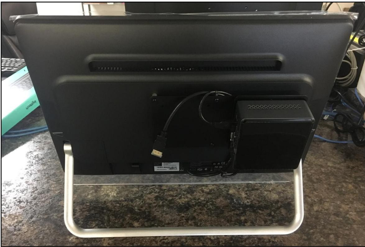
1. Plug the provided power cables into power jacks on the small CPU and the monitor and ensure that the monitor is plugged into the CPU via the HDMI cable. Plug the other end of the power cables into *Battery + Surge* side of the provided battery backup (UPS 450).
