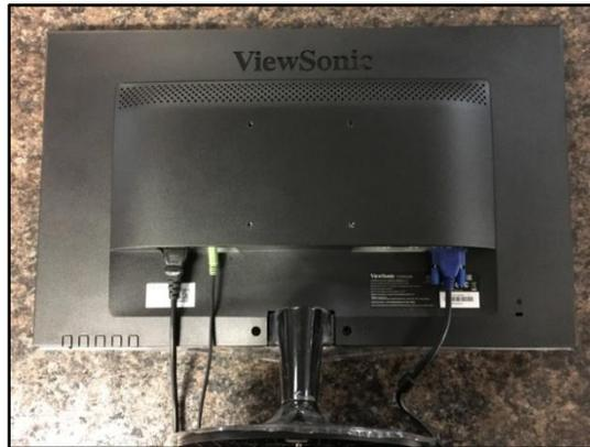
1. Plug power cord into power jack on back of monitor. Plug other end into *Battery + Surge* side of battery backup.
