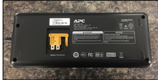
1. Turn the battery backup upside down to access the battery plug.
