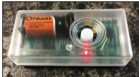
3. After 10 seconds of holding down the Alarm button, the motion sensor will start a series of initializing alarms and resets. The red LED will flash for about 20 seconds.
