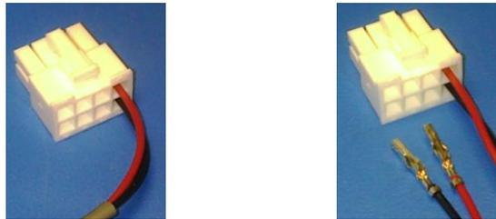
Each vertical red and black wire pairs that comes from the 24vdc power output constitutes a channel. When installing the dome lights it is recommended to balance this load by dividing the number of lights equally between the 4 channels. For VL325 series incandescent lights no more than 25 incandescent lights per channel (up to 100 lights). For VL327 series LED lights no more than 50 incandescent lights per channel (up to 200 lights).
