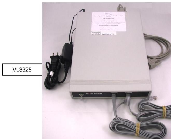
General Description: The VL3325 is an external device connected to the VisionPro console and sends alarm information to a remote monitoring station via an analog telephone line(s). It can be used in conjunction with or in place of local area pocket paging. Your dialer has been tested prior to shipment. If the phone number and account information to your Central Receiving Center was provided it was tested to YOUR Central Receiving
